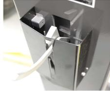
Automatic safety locks worked well, but when lift was at max rise, upon initial decent, the safety locks would have the tendency to inadvertently reset and stop downward motion on one or both sides.
