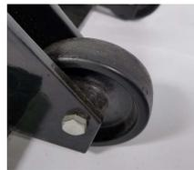
Hard, non-bearing nylon wheels did not roll well over rough surfaces.
