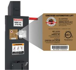
M6K models are ALI Certified. Lifts bearing the Gold Label are certified to have been tested by a Nationally Recognized Testing Laboratory (NRTL) and found to meet all industry safety and performance standards as outlined in ANSI/ALI ALCTV (current edition).
