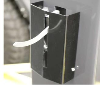
Corrected the inadvertent resetting of the safety lock(s) at full rise upon initial decent. Includes 7 safety lock positions.
