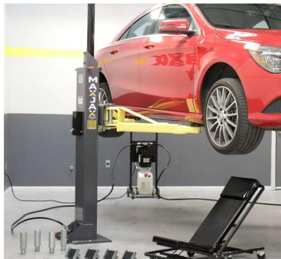
A gunmetal gray powder coat is used that has a significantly lower coefficient of friction than the textured black paint featured on previous Danmar M6 models. There is evidence that the textured paint had contributed to carriage binding problems on past units.
